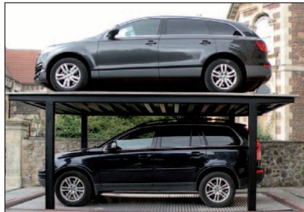
The Cardok disappears from view in the lowered position, minimising any visual impact on the surrounding area.
